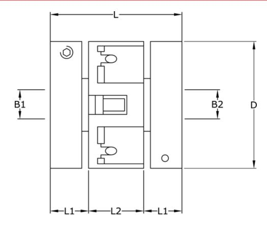
$\begin{array}{lll} B1 & = 6 \\ B2 & = 10 \\ D & = 27 \\ L & = 25.4 \\ L1 & = 9.3 \\ L2 & = 6.9 \\ Screw = M3 \end{array}$
